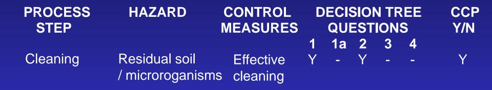
Application of the decision tree for the chemical processing stage of an endoscope. The results of the individual questions are recorded as indicated to provide transparency of decision making and can be auditable. Question 1a refers to the question "Do preventative measures exist?".
