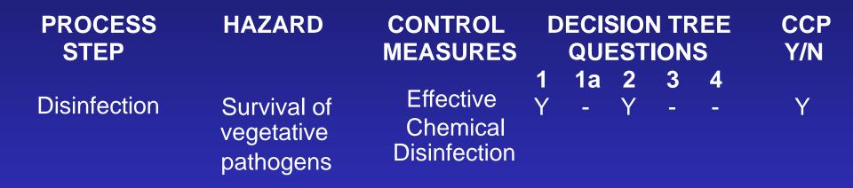
Application of the decision tree for the chemical processing stage of an endoscope. The results of the individual questions are recorded as indicated to provide transparency of decision making and can be auditable. Question 1a refers to the question "Do preventative measures exist?".
